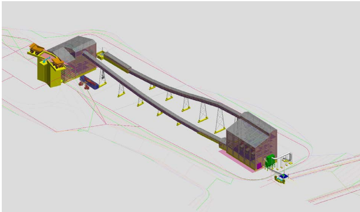
Figure 3.12: Isometric view of the Crushing and Screening Plant Layout looking southwest
