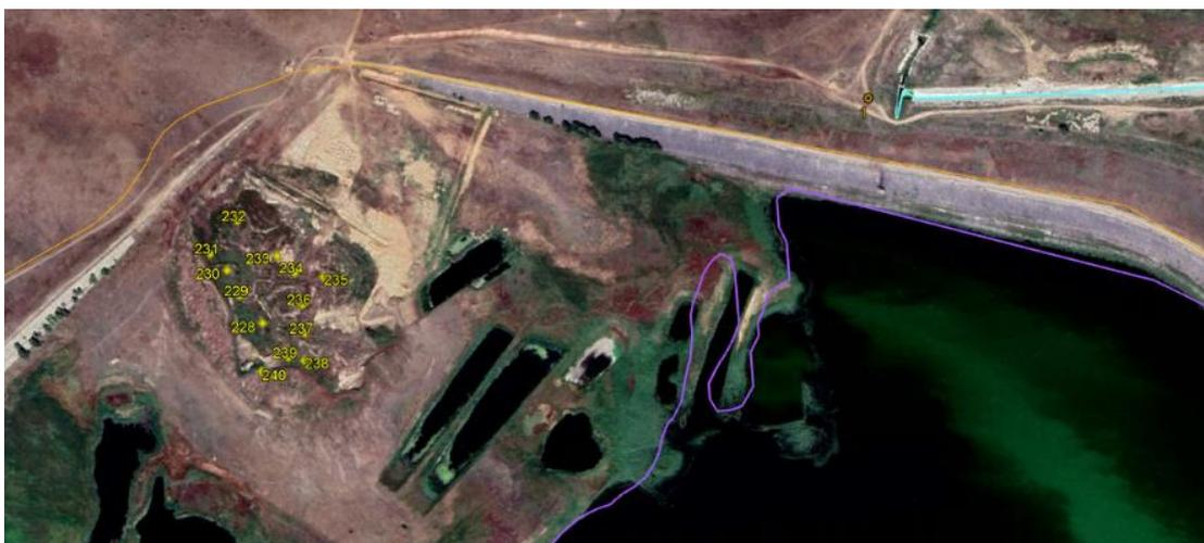
Figure 6.35: Sludge sampling points (yellow dots) within the long-term sludge storage site to the north of the URE reservoir
