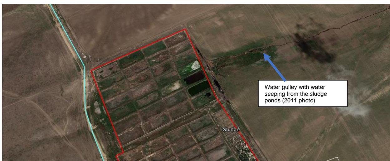
Figure 6.24 An aerial photo from 2011 showing the formation of a water gully with sludge pond water seeping into the nearby fields and towards the east.
