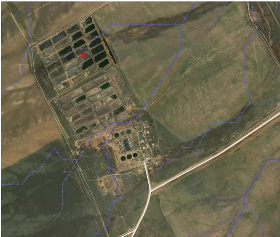
*Figure 8.3: Flow paths (blue lines) that indicate where surface runoff would pass in the area of the old and the proposed new WWTP.*
