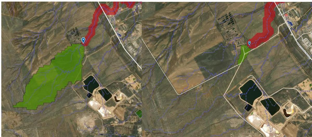
Figure 8.4: Hydrological catchment area for existing WWTP to the left and new proposed site to the right marked with green. Red marks the downstream flow path.
