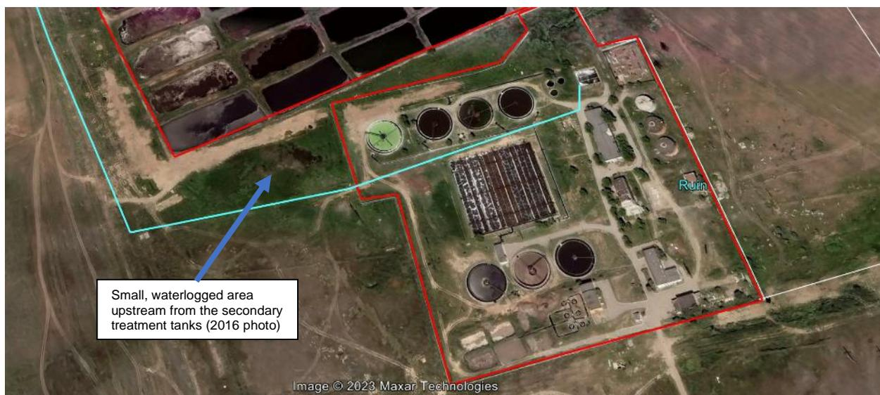
Figure 6.23 Aerial photo from 2016 showing waterlogged areas upstream from the secondary sedimentation tanks. A drainage channel was dug in 2018 to drain the resulting swamp (Map source: Google Earth, aerial photo from 8/2016)
