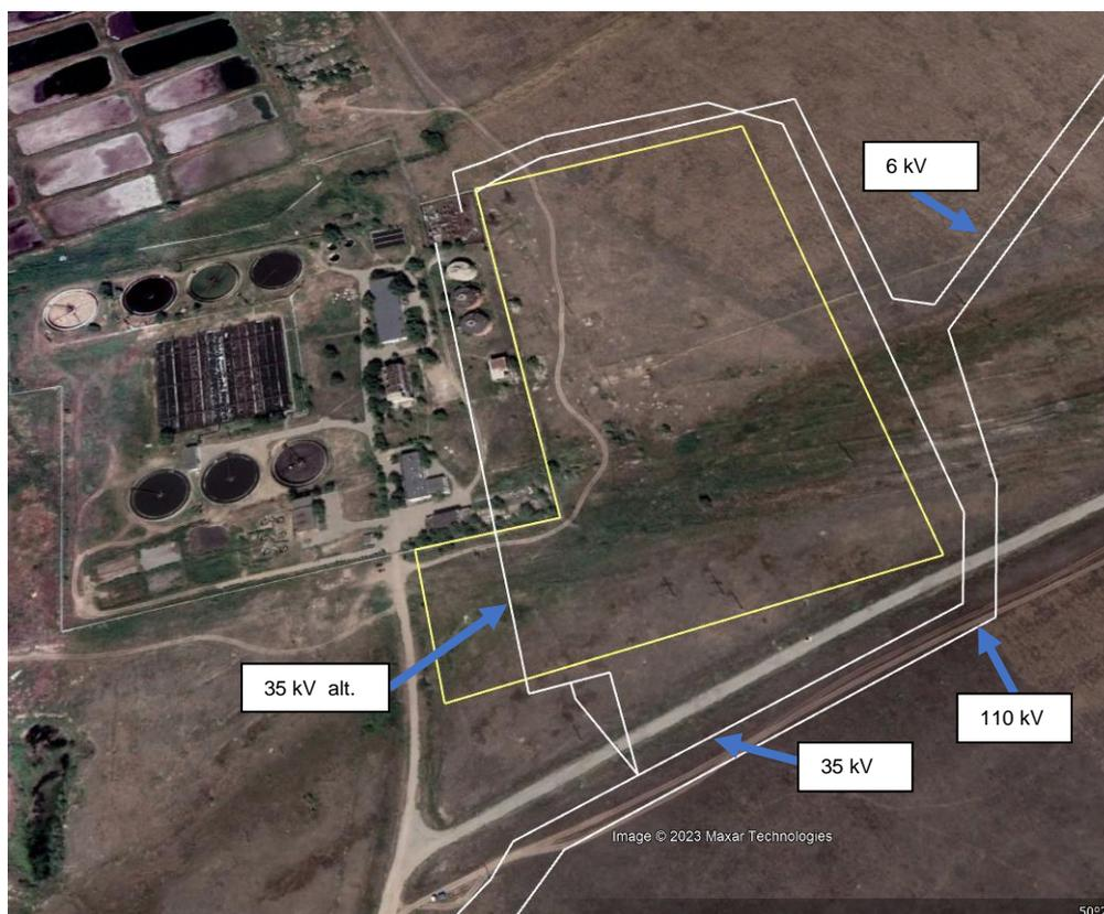
Figure 3.7 Proposed relocation of overhead lines
