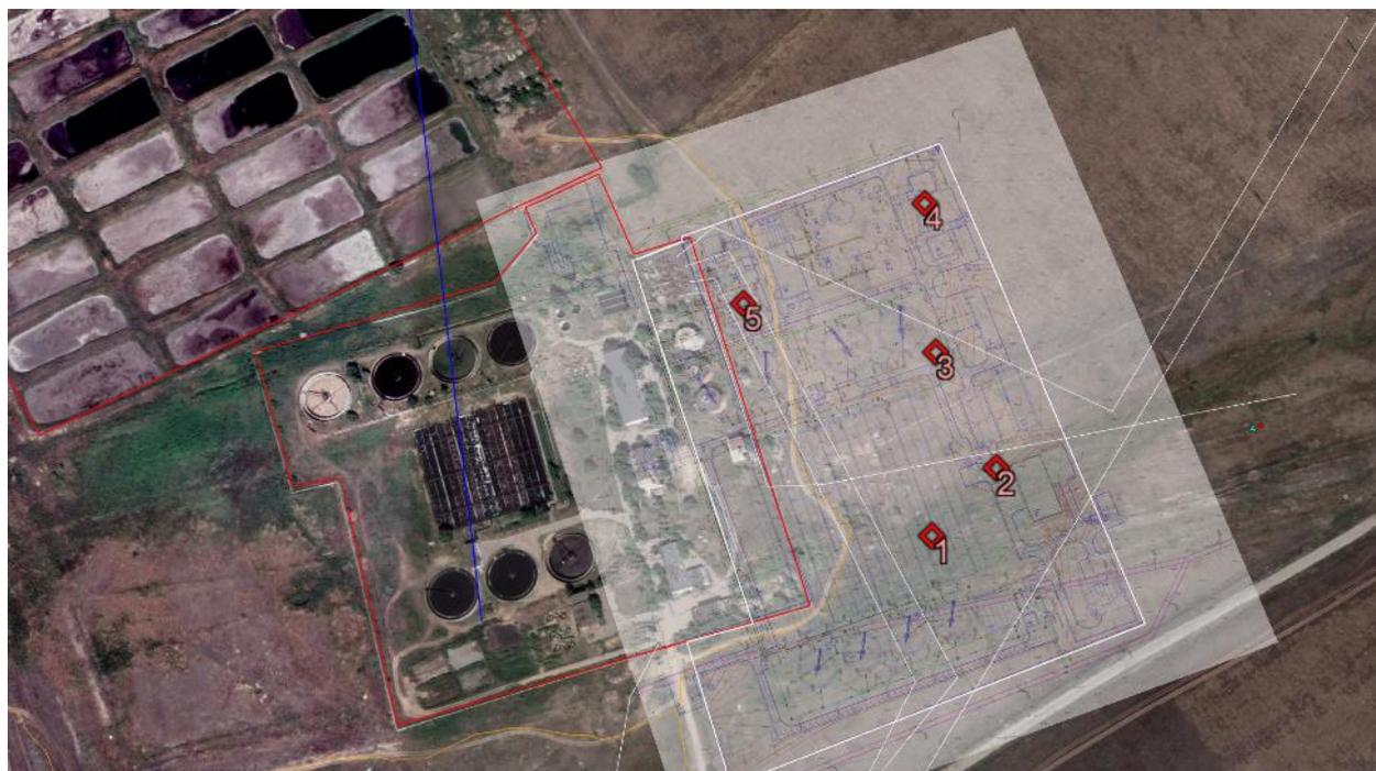
Figure 6.9: Locations of soil samples taken within the proposed WWTP site. Sampling points: 1 – lowland under planned biological tanks; 2 – lowland near the planned workshop-garage foundation; 3 – Drainage channel at the hay field edge under the planned secondary sedimentation tanks; 4 - hay field under the planned disinfection shop and 5 – a wasteland pit under the planned anaerobic digesters.
