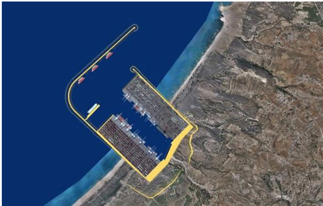
Figure 2 :Schematic view of the proposed port site and its main structures.
